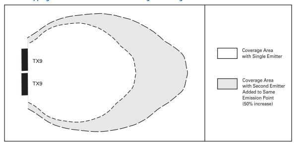
When two emitters are used at the same emission point in single channel mode, the overall coverage area increases 50%. When using an RX22-4 receiver, as a result, the coverage area will increase to an estimated 42,000 ft<sup>2</sup> (3,902 m<sup>2</sup>); the RX14-2 will increase to 5,250 ft<sup>2</sup> (488 m<sup>2</sup>); the RX16 will increase to 4,590 ft<sup>2</sup> (426 m<sup>2</sup>).
